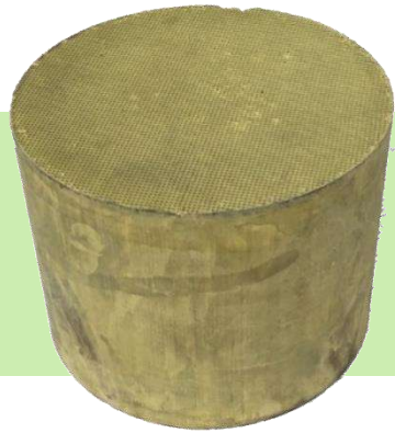
Prometheus washcoat on cordierite monoliths (400cpsi)
